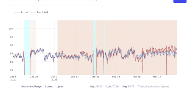
WG2 STAGEII DIS. TEMP [Asset: WET GAS COMPRESSOR PROCESS]
